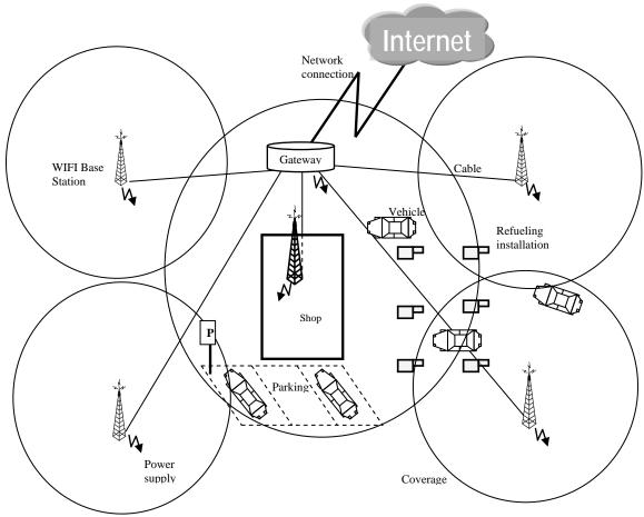
Fig. 1. Wireless LAN equipment at a service station
